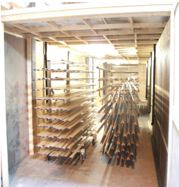
Drying chamber to maintain correct drying processes during winter months
