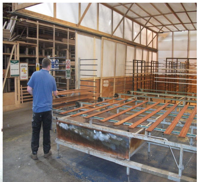
Drying chamber to maintain correct drying processes during winter months
